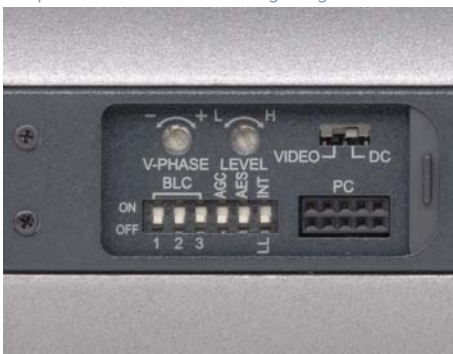
Simple DIP switches for configuring functions.
